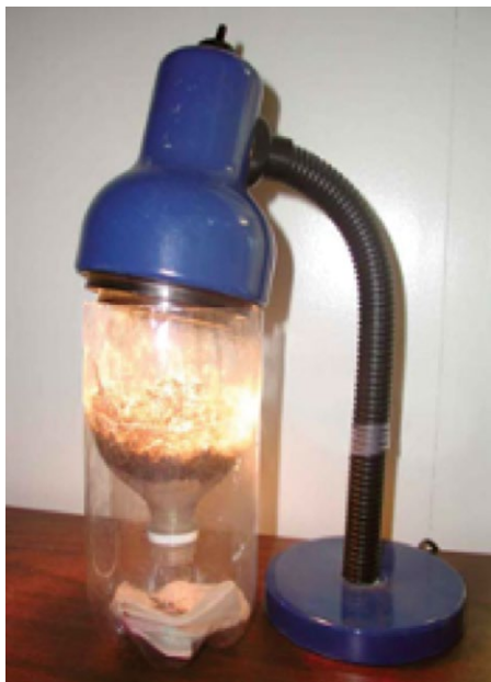
Figure 4. Berlese funnel made with a plastic soda bottle, rubbing alcohol, and a desk lamp.
