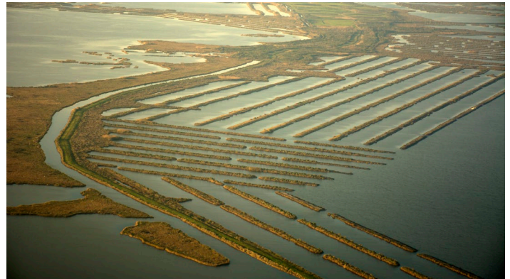
Because natural wetlands are disappearing as sea level rises, engineered wetlands are being developed in coastal Louisiana to help buffer the coast. (Lisa S. Gardiner)
