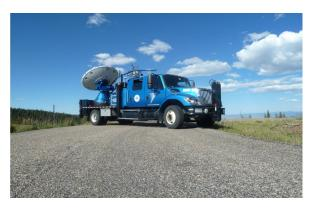
**Truck-mounted Radar:** radar mounted to the back of a truck so it can easily drive close to a storm to observe winds
