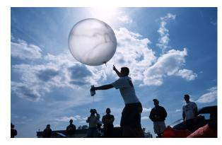
**Weather Balloon:** attached instrument measurers temperature, pressure, humidity, wind speed, & wind direction profile from the ground up to about 60,000'
